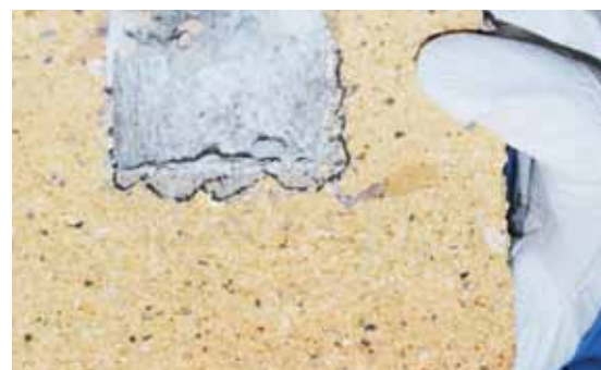
Regular test are done for measuring alkali penetration. The photo shows Bjuf SX extremely good resistance against alkali.
